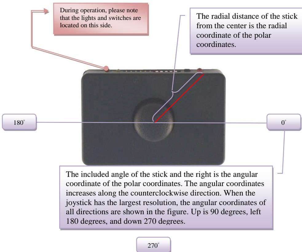
Figure 4: Joystick movements and the polar coordinate system
