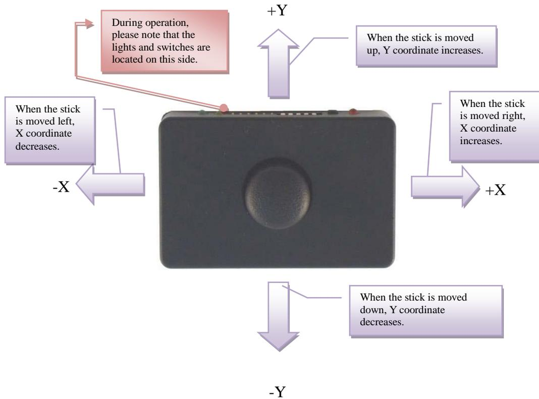
Figure 3: Joystick movements and the rectangular coordinate system
