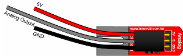
Figure 3 TCRT5000 Board connection for analog output
