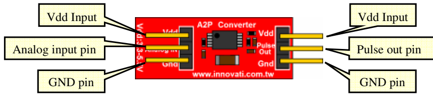
Figure 2 A2P Component Description
