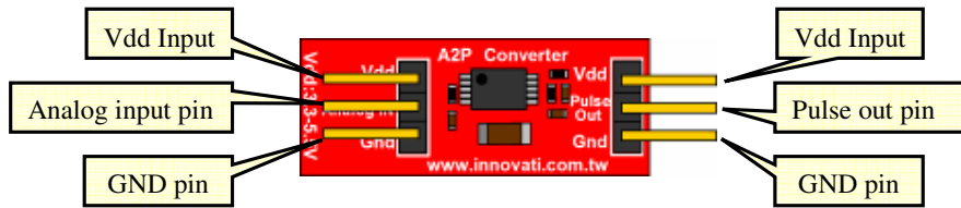
Figure 2 A2P Component Description
